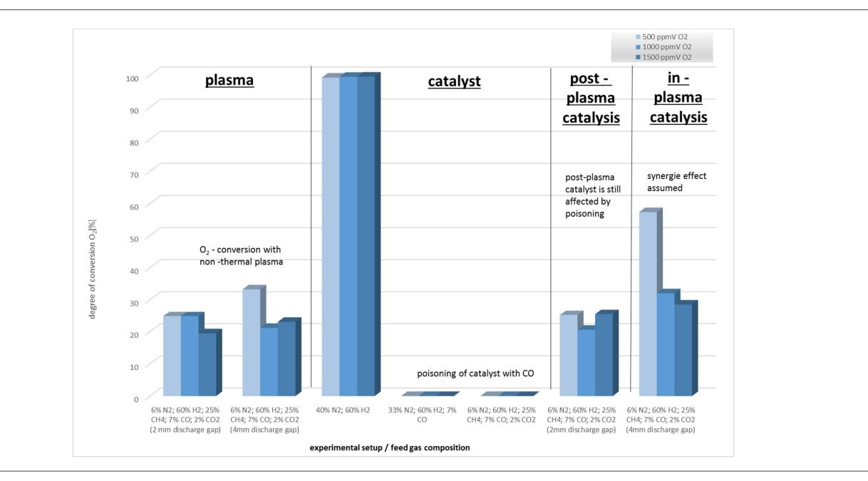
Figure 2: results of  $O_2$  conversion in model steel mill gas
